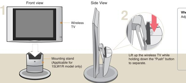
When watching the wireless TV using the mounting stand Adjust the angle of the stand as shown below.
